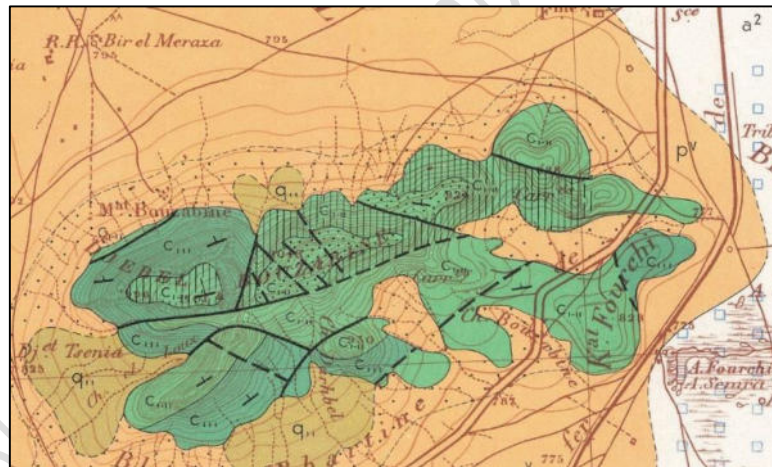
Figure 6 : Extract of a geologic map showing depositional contacts (continuous or dotted thin lines) and fault lines, visible or not (continuous or dotted thick lines).
